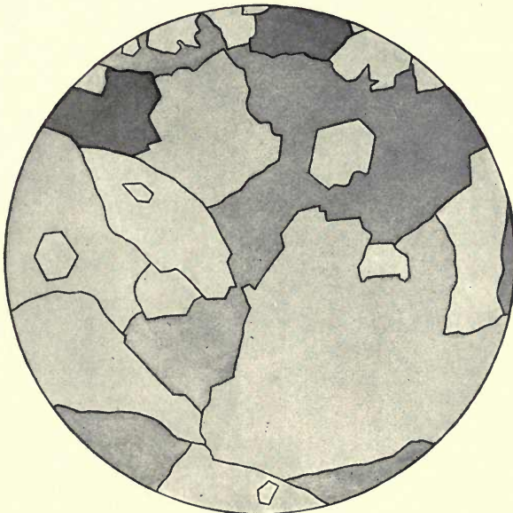
Primary Vein Quartz from Filling. Federal Loan mine, Nevada county, Cal. Crossed nicols. All Quartz. Magnified 14 diameters.
